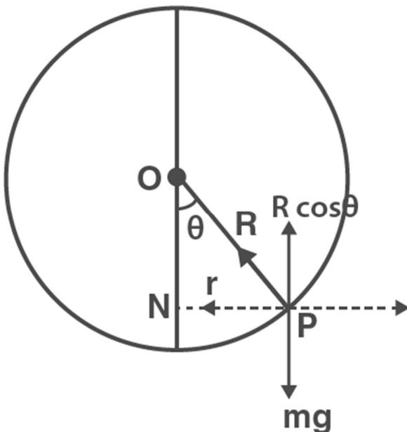
Let  $\theta$  be the angle made by the radius vector joining the bead and the centre of the wire with the downward direction. Let,  $N$  be the normal reaction
